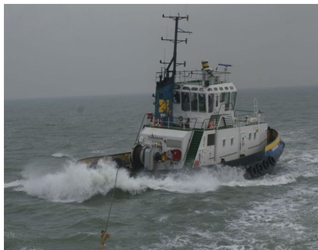
Fig. 10 : Dynamic sea tests, SafeWinch cuts off peak loads and prevents slack wire
